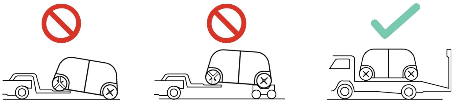
8. Safely secure the robotaxi to the bed of the truck using the strap tie down method around the wheels. Once secure, release the tension from the winch cable and remove the wheel skates.
