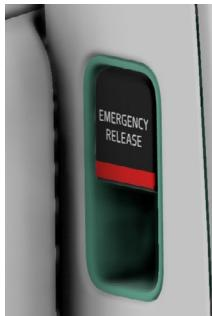
There are 2 release handles on opposite sides of the robotaxi rider cabin, one for each set of doors. When facing the door from the robotaxi exterior, the handle is on the right side.
