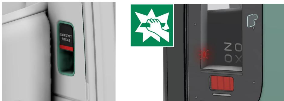
2. Pull the Emergency Release handle to a 90 degree angle to release the door latch. The door latches release and if power remains, the system attempts to open automatically. Step back from the robotaxi as the doors open. If no power remains, the handle will need to be held in the pulled-up position while the right-side door is opened manually.
