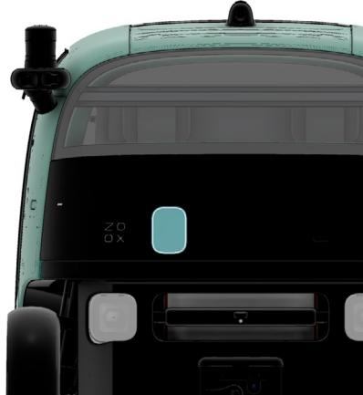
The following documents can be found in a document clip, placed inside the Chargeport door. The Chargeport door can be unlocked remotely by Zoox Remote Operators. If they are unable to assist, on-site Zoox Support Team members will be able to unlock the Chargeport door:
