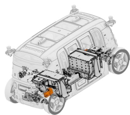
The AC Compressor is powered by the HV system. Zoox robotaxis have 2 AC compressors on the robotaxi, 1 within each drive module. Within their respective drive module, they are connected to the HV battery through an HV cable.
